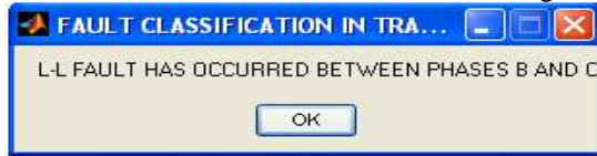
Fig. 15 Matlab Result for LL Fault
